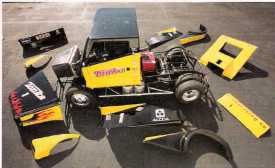
■ It looks like a standard road truck, but it's built like a race car. Steel tube space frame with fiberglass body panels is powered by a 14,000-cc Detroit Diesel turbo 6-cylinder engine with 2200 lb.-ft. of torque!
